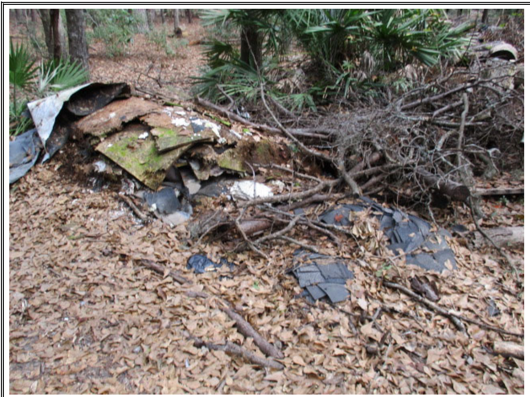
Photo No. 8: Example solid waste debris observed at project site (laboratory analysis confirms roofing shingles do not contain asbestos).
